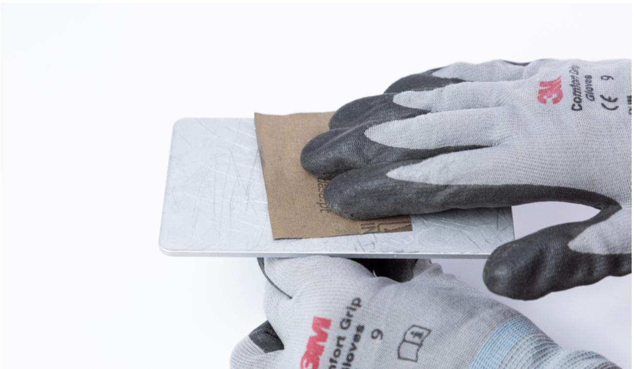
3. While preparing your model in Z-SUITE, follow the steps from this article: <https://support.zortrax.com/inkspire-model-orientation-supports/>. Also, to improve the model's adhesion during the printing process, polish the platform's surface with sanding paper.
