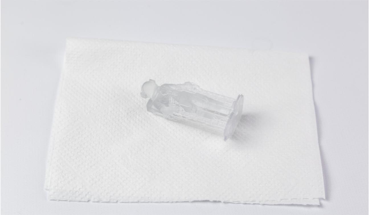
5. After final rinsing, make sure to dry the print completely.
