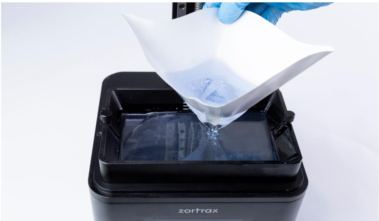
2. Pour the resin into the tank and wait until there are no air bubbles in the liquid. Air bubbles can get printed into the model and influence its aesthetics negatively. To speed this process up, pour the resin through the resin filter.
