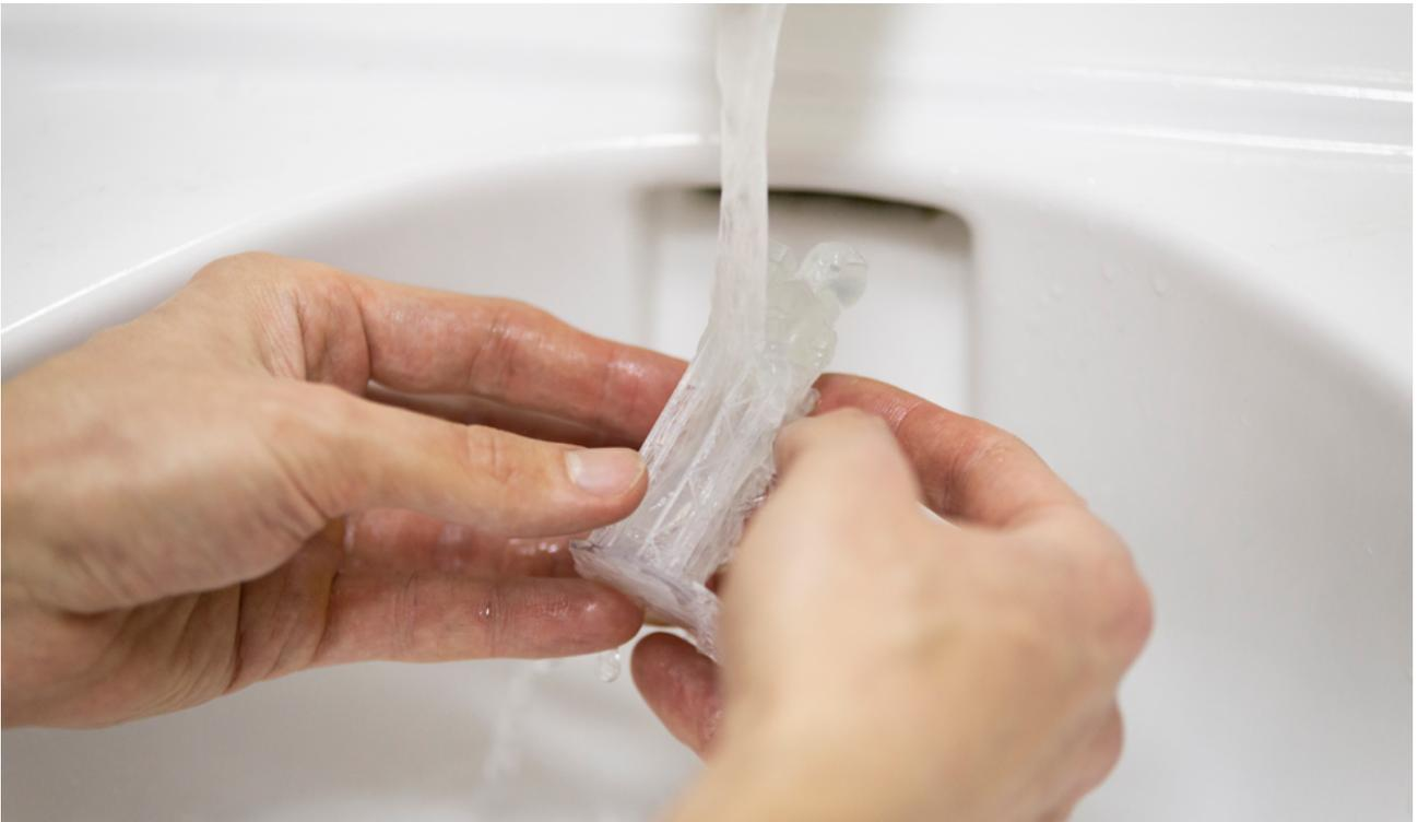
4. Put the ready print into an IPA bath for 3-5 minutes. Next, rinse the model with lukewarm water and then leave it to air dry. Repeat these steps three times.
