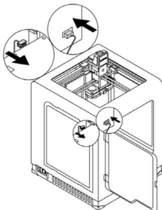
11. Plug the heatbed cable into the platform and into the adapter placed in the Z-axis cover.
