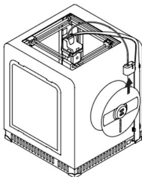
17. Feed the material into the extruder through the material endstop and the material guide.
