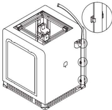
12. Install the extruder cable clamps in the holes at the back of the printer. Place the extruder cable in the clamps.
