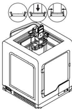
13. Remove the extruder top cover and plug in the extruder cable.
