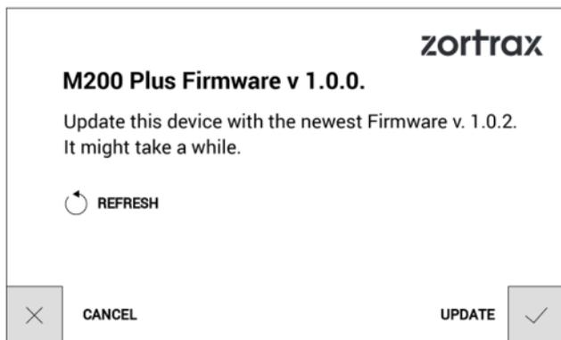
If you have decided not to connect the printer to the Internet, check <https://support.zortrax.com/downloads/> regularly for updates. To update the firmware, transfer the Update.zar file to a USB flash drive and plug it into the port at the front of the device. To start the installation, select *Refresh*.
