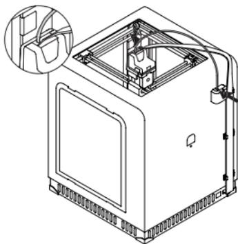
15. Attach the material guide to the extruder and to the material endstop.
