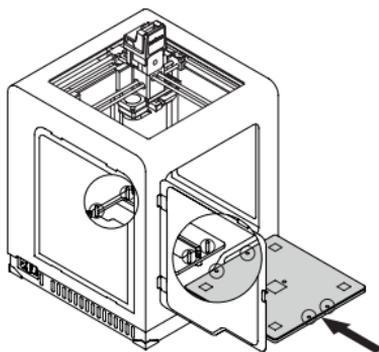
10. Install the build platform onto the bolts marked in the picture. Remember to install the platform with the perforated plate with its five silver calibration squares directed up.
