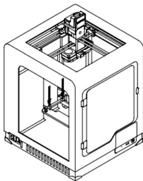
8. Lower the heatbed mount by pressing the places marked in the picture.
