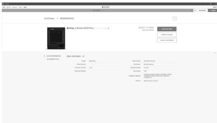
Each added printer can easily be managed in Z-SUITE. You can start, stop, and pause the printing process, see the printer's current state (*Ready to Print / Printing / Paused / Offline*), change the name of your printer, preview basic information about the printer, or display the preview from the printer's camera.
