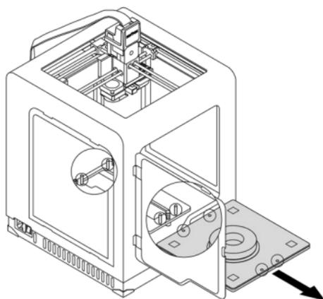
4. Remove the platform from the printer.
