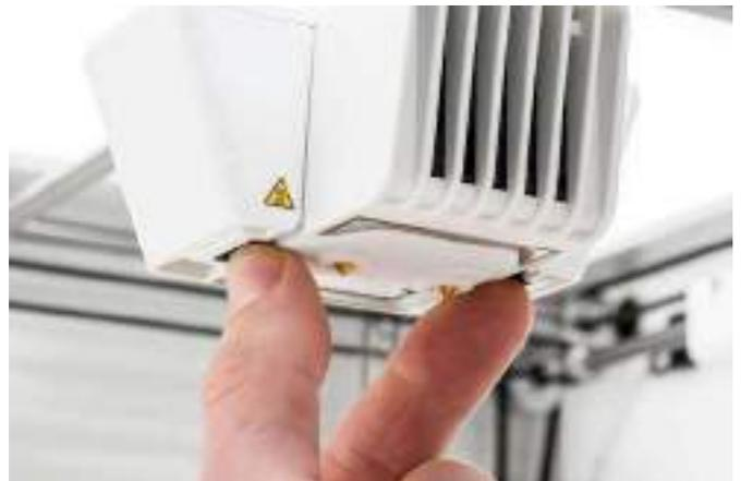
LE CAPOT DE BUSE NE DOIT PAS SE DETACHER FACILEMENT DU SUPPORT DE VENTILATEUR
